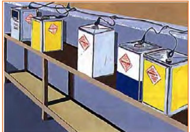
Fig.3.1.15: Earthed containers to store flammable solvents
