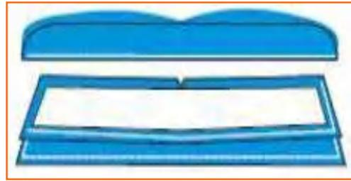
**Step 4:** Take the other neckband piece without fusing. Place it below the ready neckband collar piece.
