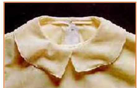
Fig.2.3.13(c): Interlining shrinking
