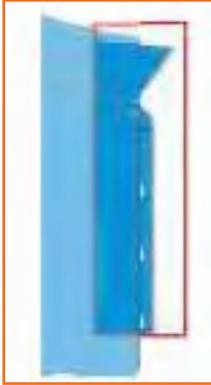
**Step 1:** Keep the left hand and right hand plackets on top of each other. They should be properly aligned.
