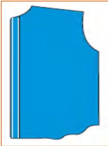
**Step 7:** Again from the bottom, stitch the outer side of the placket using edge stitch.
