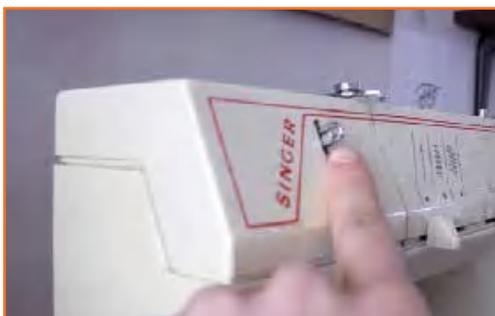
**Step 5:** Then bring it down from the take up lever into the coiled thread guide.
