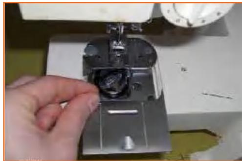
**Step 9:** Pull the string out tight and set the bobbin into the tray. Insert the thread into the metal notch and pull back.
