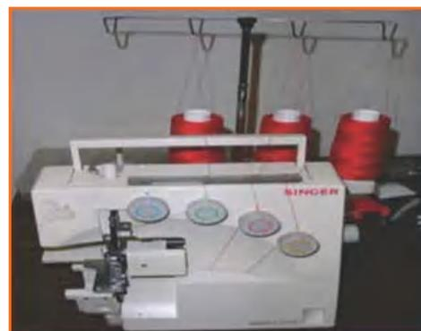
Fig:4.1.4: Over lock / over edge machine
