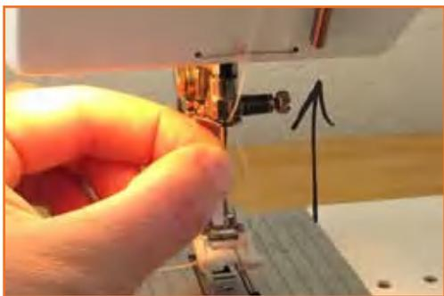
**Step 3:** With the flat side towards the back, push the new needle up inside the needle clamp as high as it will go.
