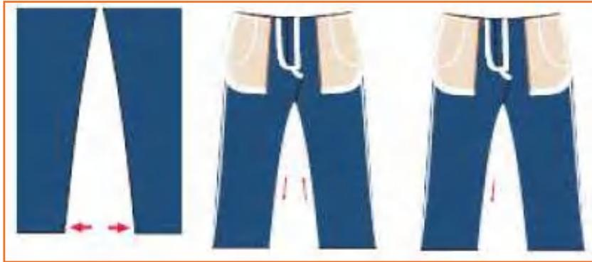
**Step 5:** Put 5-thread overlock stitches starting from bottom to finish at other bottom side.
