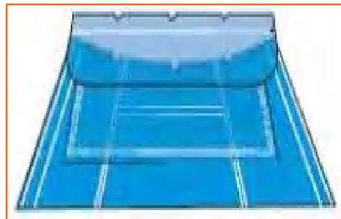
**Step 2:** Keep the left hand side with face up on the Fig. Match the edge of the front placket with the edge of the collar band.
