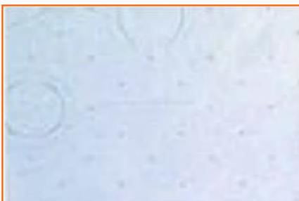
Fig.2.3.13(a): Ideal fusing in fabric
