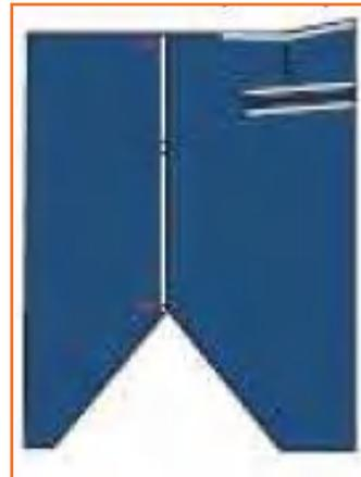
**Step 4:** Turn the raw edges towards the left side and put top-stitch at the edge of the back rise.
