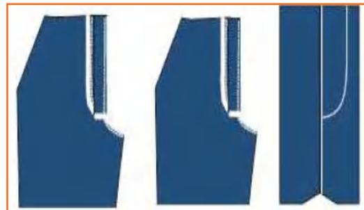
**Step 19:** Turn the piece so that the front side of the fabric is facing up. Put an edge stitch on front rise starting from bottom till the end of J-stitch.
