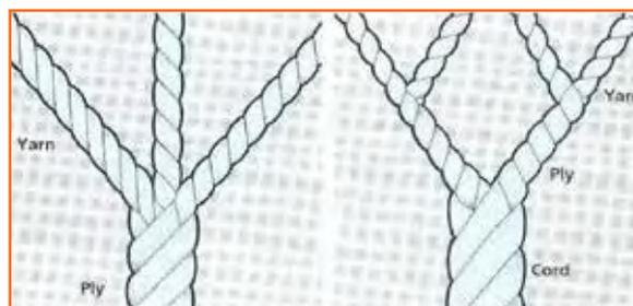
Fig.2.5.26: Ply and Cord of Thread
