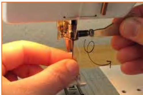
**Step 1:** Hold the needle with your left hand and undo the screw at the top of the needle with your right hand.
